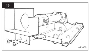
9.4 Refer to the technical specification and databadge to check the gas type and its required aeration plate. Change the aeration plate, if necessary.
